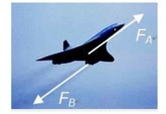
$F_A$  = force exerted on the plane by the ejected gas
